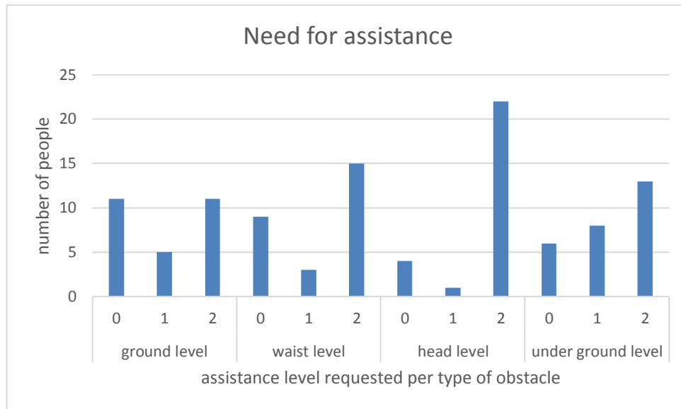
The most important kind of obstacles is by far head level obstacles (tree, ladder, scaffolding, etc.). Indeed, these obstacles cannot be detected by the standard white cane (even by a guide dog in most cases) while they can be very painful when hit. An assistance is also widely asked for the waist level (work barriers, truck back, restaurant tables) and the underground obstacles (holes, steps down, fountains, manhole cover).
