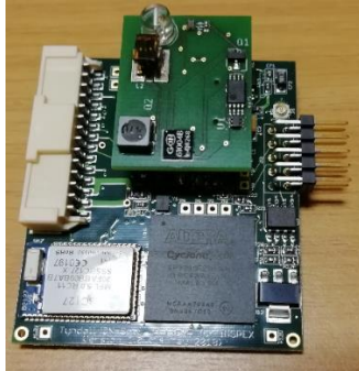
Figure 5: Long range LiDAR module (optic board on top of mother board) Figure 6: Short Range LiDAR
